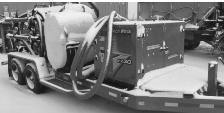
VACUUM UNIT USED TO RECOVER CONTAMINATED WATER AND SOLIDS.
