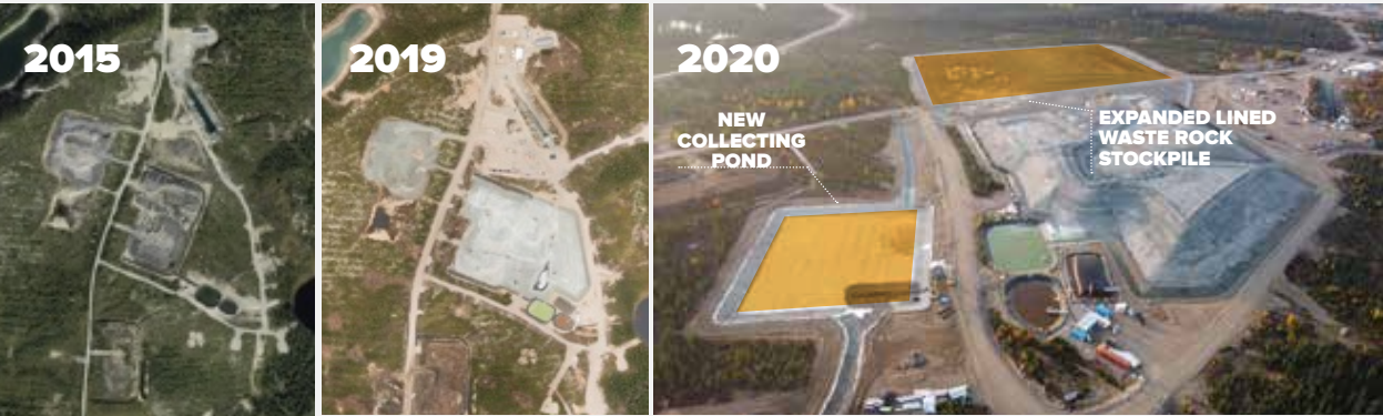
The evolution of the lined waste rock stockpile and the water management system (2015, 2019, 2020).
