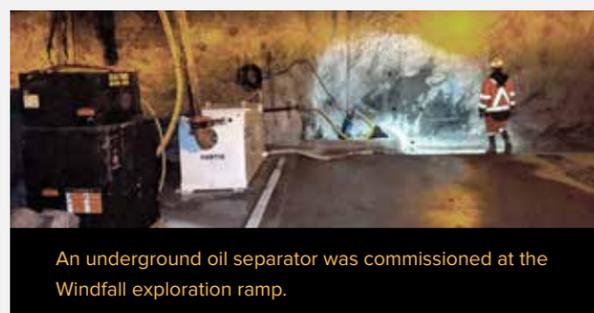
An underground oil separator was commissioned at the Windfall exploration ramp.
