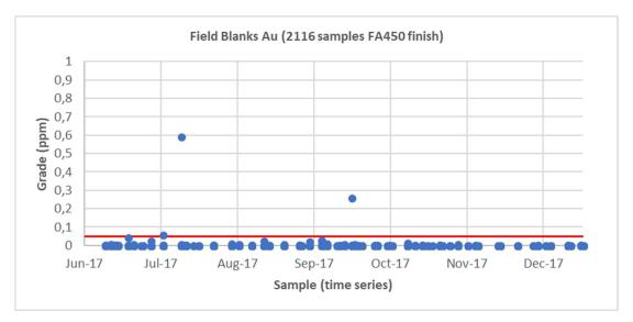
Detection limits set at 0.05 g/t Au (10x detection limit)
