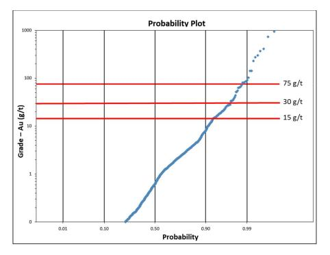
Figure 14-5: Example of four-step gold grade capping on composites from the major zones in Z27 area using a probability plot of grade distribution
