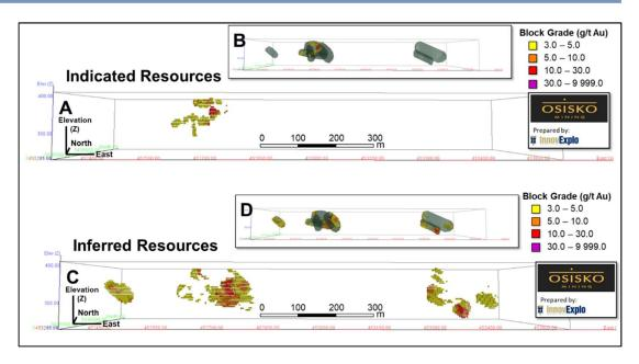
A) 3D view looking north and B) 3D view looking NW showing indicated resources (>3.0 g/t Au) inside the zones; C) 3D view looking north and D) 3D view looking NW showing inferred resources (>3.0 g/t Au) inside the zones.
