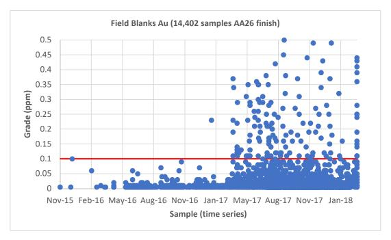
Figure 11-2: Time series plot for blank samples assayed by ALS (AA26 method). Detection limits set at 0.1 g/t Au (10x detection limit)
