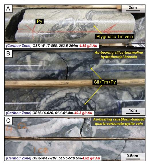
A) A ptygmatic tourmaline and Fe-carbonate vein in disseminated to semi-massive pyrite. B) Low-angle goldbearing silica-tourmaline hydrothermal breccia. C) Low-angle gold-bearing crustiform quartz-carbonate-pyrite veins. All gold grades (Au g/t) are cut to 100 g/t unless indicated
