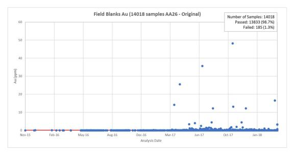
Figure 11-5: Original blank results for AA26 method with statistics Detection limits set at 0.1 g/t Au (10x detection limit)
