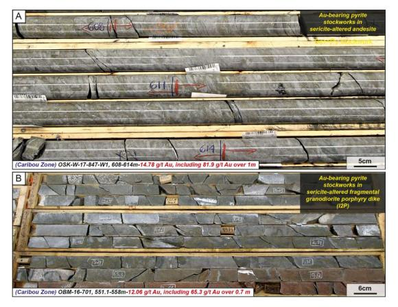
A) Pyrite stringers associated with strongly sericite-altered andesite. B) Strong sericite alteration associated with gold-bearing pyrite stockworks at the contact between a fragmental granodiorite porphyry dike (I2P) and a red quartz-monzonite (Red Dog). All gold grades (Au g/t) are cut to 100 g/t, unless indicated.
