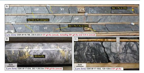
A) Silicified and strongly sericitized rhyolite containing abundant pyrite stringers and local specks of gold in contact with porphyry dikes (I1P). B) Bonanza-grade zone associated with strong silica-pyrite alteration. C) Goldbearing silica-tourmaline hydrothermal breccia. All gold grades are cut to 100 g/t unless indicated.
