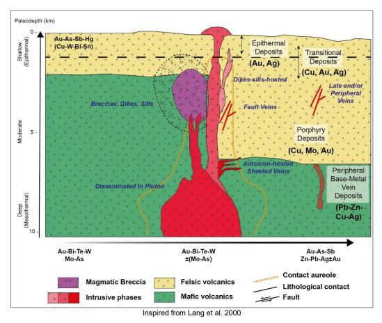
Figure 8-1: Schematic geological model for intrusion-related gold systems at Windfall showing lateral and vertical mineralogical zonations
