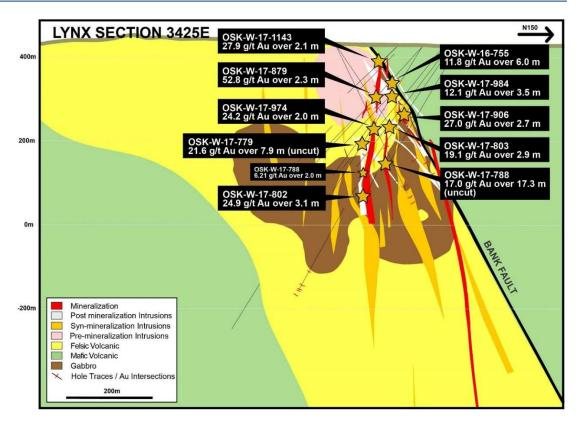
Figure 10-2: Representative geological cross-section showing the distribution of drill hole spacing and orientation and significant assay results in the Lynx zone (section 3425E)
