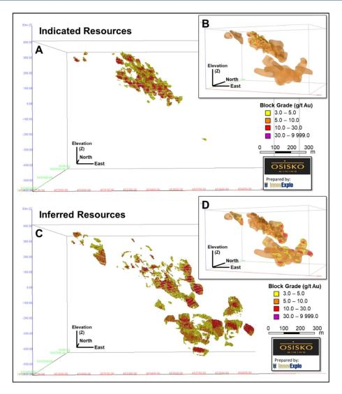
A) 3D view looking north and B) 3D view looking NW showing indicated resources (>3.0 g/t Au) inside the zones; C) 3D view looking north and D) 3D view looking NW showing inferred resources (>3.0 g/t Au) inside the zones.
