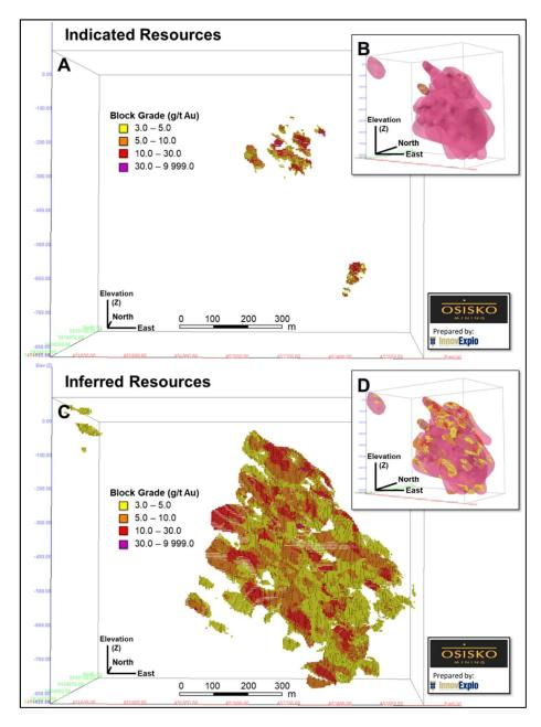
A) 3D view looking north and B) 3D view looking NW showing indicated resources (>3.0 g/t Au) inside the zones; C) 3D view looking north and D) 3D view looking NW showing inferred resources (>3.0 g/t Au) inside the zones.
