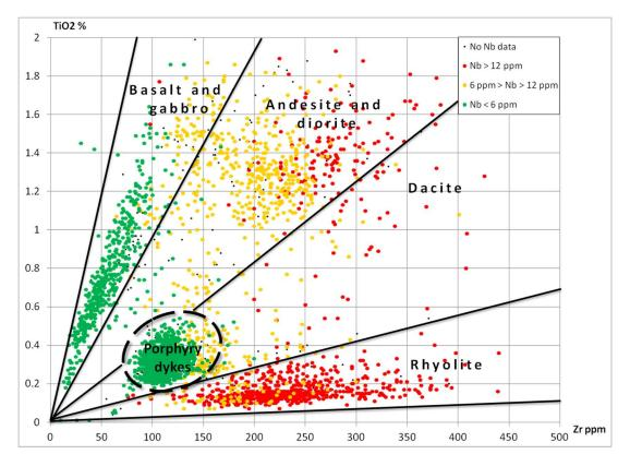
Figure 7-6: Discrimination of rock units on a TiO<sub>2</sub> vs. Zr diagram with Nb values in coloured dots
