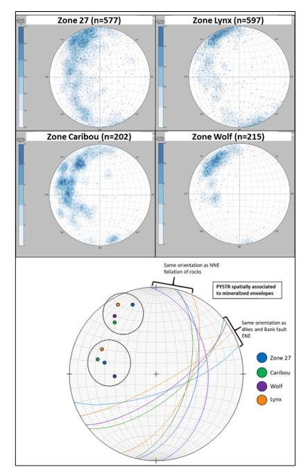
Figure 7-18: Stereographic projection of pyrite stringers (PYSTR) proximal to mineralized envelopes from Zone 27, Caribou, Wolf and Lynx along with the interpretation
