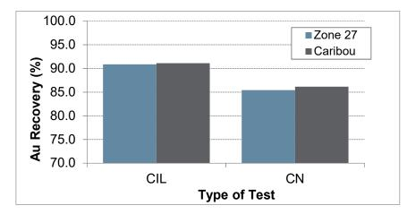
Figure 13-10: Gold recovery from CIL vs. cyanidation without carbon (at 72 hours)
