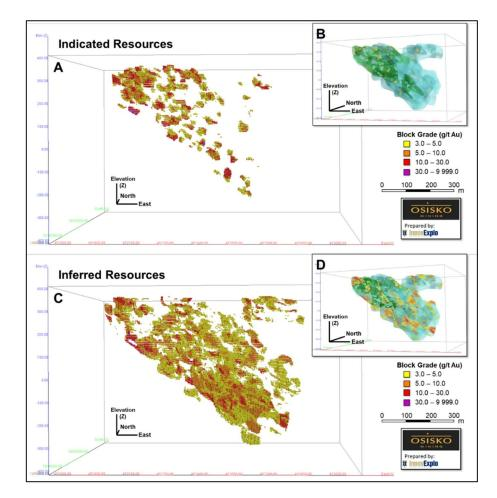
A) 3D view looking north and B) 3D view looking NW showing indicated resources (>3.0 g/t Au) inside the zones; C) 3D view looking north and D) 3D view looking NW showing inferred resources (>3.0 g/t Au) inside the zones
