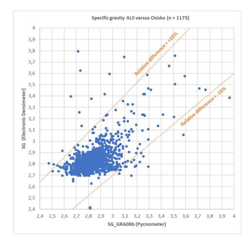
Figure 11-10: Lab (GRA08b) and internal specific gravity (SG) measurement correlation (Eagle Hill and Osisko)
