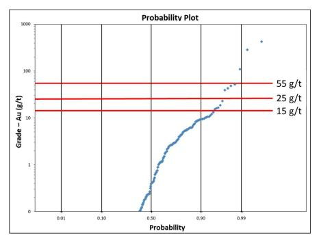
Figure 14-8: Example of four-step gold grade capping on composites from all zones for F Zones area using a probability plot of grade distribution
