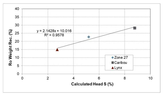
Figure 13-6: Rougher weight recovery vs. %S in feed
