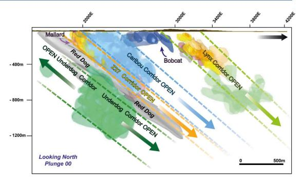
Figure 7-10: Leapfrog 3D modeling illustrating idealized vertical cross-sections (looking North) of the geometry of the mineralized zones plunging 30° to the NE (Caribou, Zone 27, Underdog, and Lynx zones). The Mallard and Bobcat zones are indicated by the purple and dark blue arrows, respectively. Exploration is open at depths for all zones. The Underdog zone is also open up-plunge for exploration.
