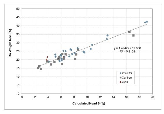
Figure 13-8: Rougher weight recovery vs. %S in feed
