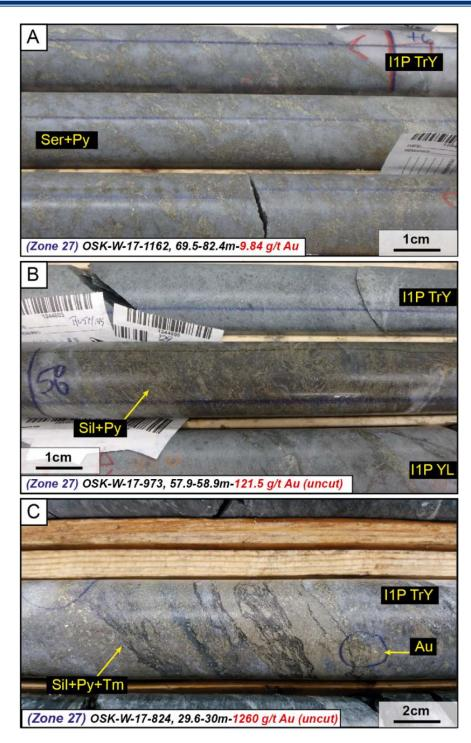
A) Pyrite stringers associated with strong phyllic alteration within a quartz-feldspar porphyry dike (I1P TrY). B) Strong silica alteration associated with gold-bearing pyrite mineralization at the contact between two phases of quartz-feldspar porphyry dikes. C) Visible gold associated with abundant pyrite and tourmaline mineralization in a strongly silica-sericite altered quartz-feldspar porphyry dike. All gold grades (Au g/t) are cut to 100 g/t unless indicated.
