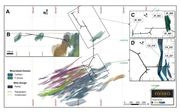
A) Plan view; B) Cross-section looking east; C) and D) 3D close-up views of F Zones and Caribou corridor
