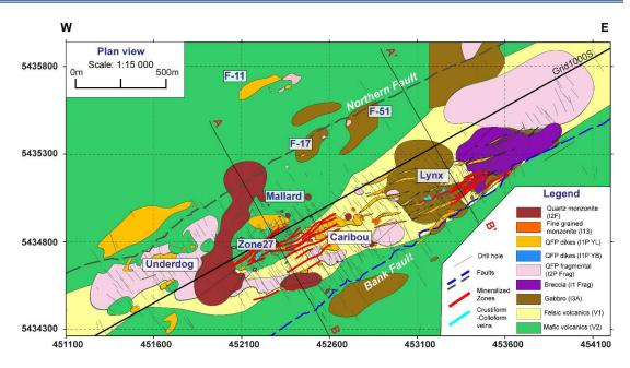
Figure 7-8: Interpreted surface geology of the Windfall Lake gold deposit with logged mineralized zones and lithologies projected to surface illustrating the spatial relationship between syn-mineral I1P dikes (orange) and gold mineralization (red). Refer to Figure 7-9 and Figure 7-14 for vertical cross-sections (A - B "Main zone") and (A'- B' "Lynx zone").
