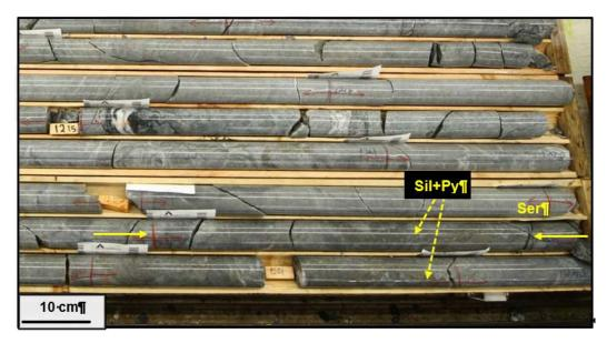
Figure 7-13: Drill hole OSK-W-17-821-W1. Strong sericite with localized zones of strong silica alteration coupled with pyrite-gold mineralization within a synmineral quartz porphyry dike (I1P) in the Underdog mineralized zone. The average gold assays from 1,219.4-1,220.1 m (marked by solid yellow arrows) is 13.75 g/t gold (cut to 100 g/t).
