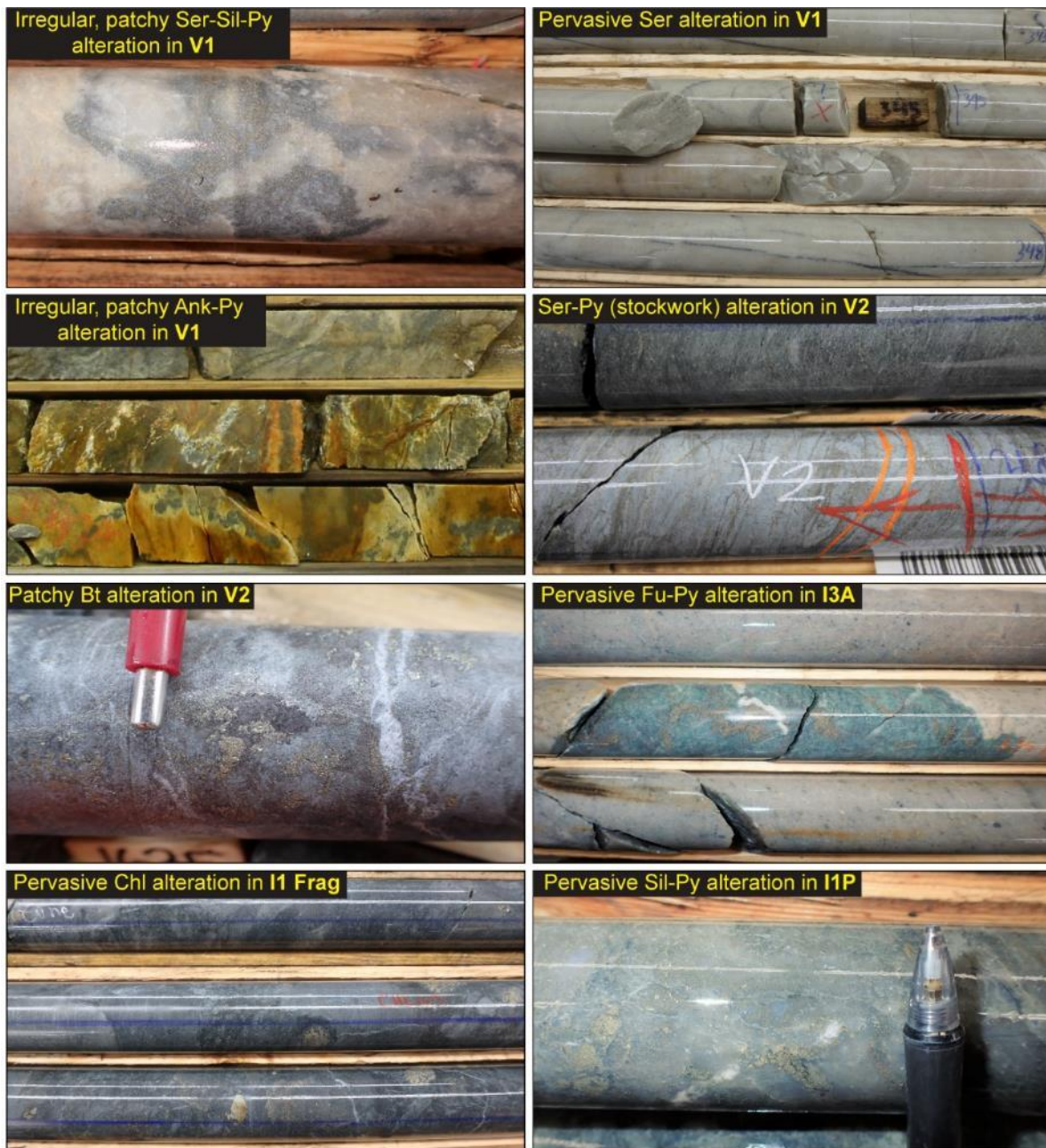
Figure 7-3: Visual alteration assemblages observed in drill core at the Windfall deposit
